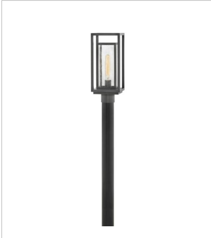
1001OZ-LV MEDIUM POST TOP OR PIER MOUNT 7" W, 17" H Socketed 1-3.50w Med. LED *Included
